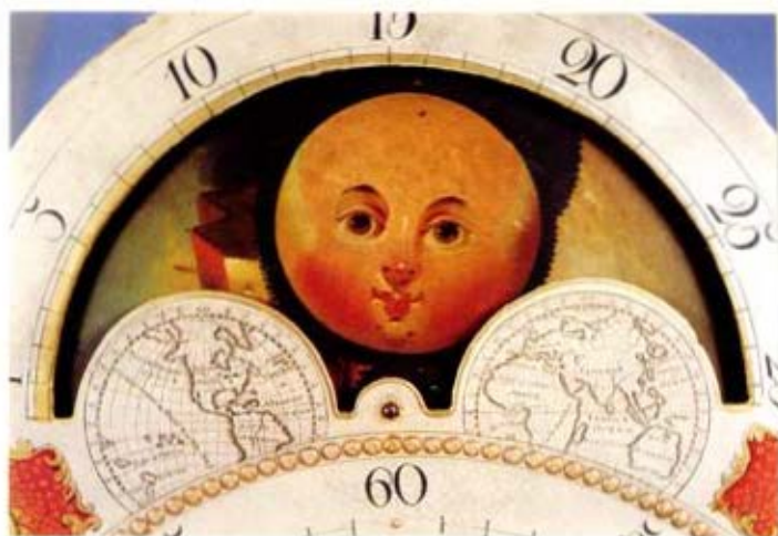
Figure 10. Spencer Nolen dial hemispheres c. 1810—1815; these hemi- spheres have lati- tude markings every 10 degrees and no ecliptic.
